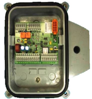
ESD module in the cable distribution box
