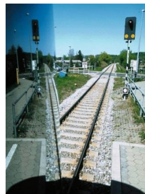
Signal indication BÜ1 on a repeater signal
